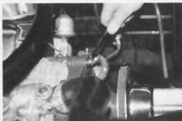
The supercharger mounting bracket is next. Remove the two cap screws from the water pump...
