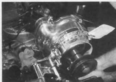
Next, Glenn bolted the Paxton Novi G.S.S. supercharger housing into place.
