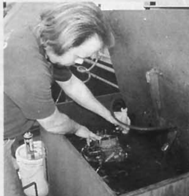
Meanwhile, it was back over to JET, where technician Sean Murphy began the fuel delivery system modifications by thoroughly degreasing the carburetor.
