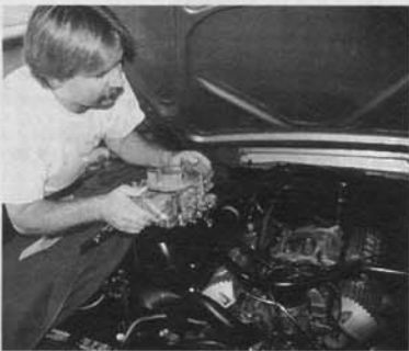
Once the battery has been disconnected, the radiator overflow and windshield wiper reservoir can be removed along with the Mustang's 700-cfm Holley carburetor.
