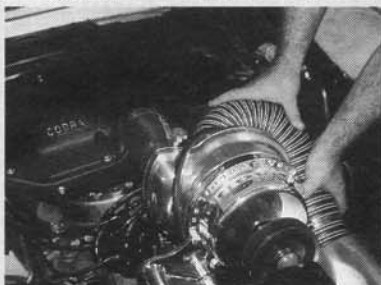
It was now time to bolt on the top of the carburetor bonnet and connect the Paxton's air inlet hoses.
