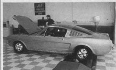
After a quick (mighty quick, from our vantage point in the copilot's seat!) test drive around the block, the Mustang was put on the dyno rollers at JET once again. With the Paxton generating 6-pounds of manifold pressure, the Mustang registered 447 horsepower at the rear wheels. That's a whopping 129 horsepower increase at the rear wheels! Not bad at all for an afternoon's worth of labor.
