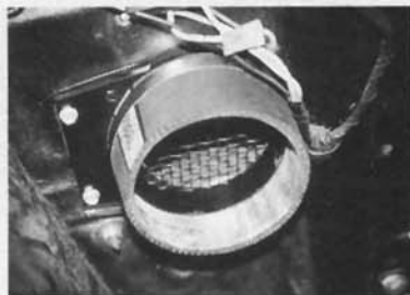
A trial fitting of the air cleaner screen revealed some slight interference with the freshly relocated voltage regulator. The problem was easily remedied by rotating the voltage regulator 90 degrees.
