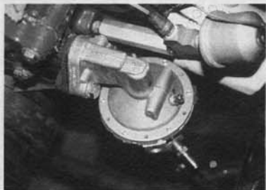
The high-volume fuel pump is bolted in place using the 1/4-inch Grade-8 bolts supplied in the kit.
