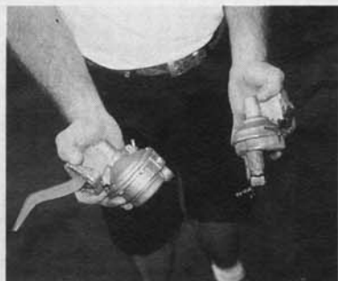
Fuel enrichment would be a major concern when under boost, so the Mustang's Carter mechanical fuel pump was replaced with a new version. The new Carter pump, on the left, which is supplied in all of Paxton's kits, utilizes a vacuum fitting located on the top of the pump body to sense supercharger boost, then spikes the fuel pressure to stave off detonation.
