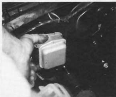
From there, it was on to mounting the Paxton's special air filter element, which is encased in a custom aluminum housing. But first, the factory voltage regulator must be relocated 4.5-inches above its original position on the front support.
