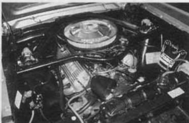
The Wheeler Speed Shop-built 289 small-block nestled between the framereils of Rich Fabbri's '66 Mustang fastback generated 318 horsepower on Jones Electronic Technologies' chassis dyno in normally aspirated form. How much power can it generate when its cylinders are pressurized with 6 to 7 pounds of boost from the Paxton Novi G.S.S. centrifugal supercharger? Keep reading to find out.
