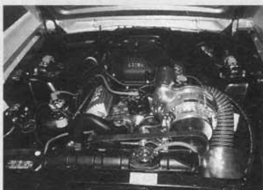
The final steps before fire up were to reinstall the distributor and attach the vacuum/boost line from the supercharger housing to the boost-sensitive Carter fuel pump. Garcia also bent a custom fuel line from the pump to the carburetor to clear the supercharger housing's large inlet.
