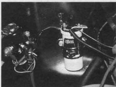
With the large amounts of air and fuel that would be force-fed into the 289's combustion chambers, Glenn decided to add a high output ignition system. The ACCEL coil, which now resides on the passenger side inner fender well, fits the bill nicely.
