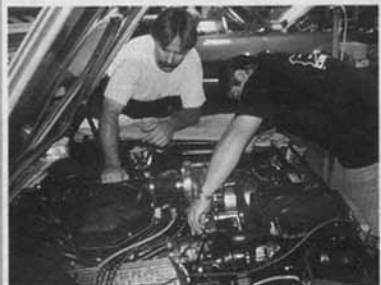
Finally, the supercharger belt is installed, Garcia then set the timing at 8 degrees initial advance while Gruettke checked for any vacuum or fuel leaks.
