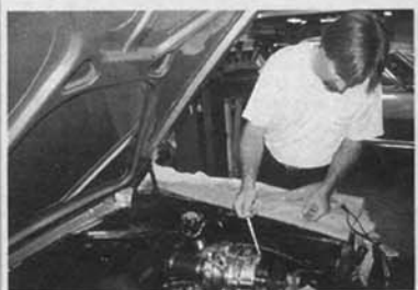
It's now time to add the lubricating oil to the supercharger housing. Glenn added the recommended 8 to 10 ounces of Paxta-Trac synthetic fluid to the blower, insuring proper lubrication. Paxton recommends that fluid levels be checked at regular intervals, as well.
