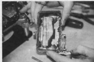
The factory Holley floats are not up to the increased fuel pressures associated with forced induction applications, production pieces will collapse under that pressure. So...
